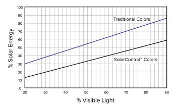
Note: Both Polycast SolarControl<sup>™</sup> materials transmit high amounts of visible light (400 to 700 mm) and transmit much less radiation in the near-infrared (NIR) and in the UV. The NIR and UV regions contain significant amounts of solar energy, but do not contribute to visibility.
