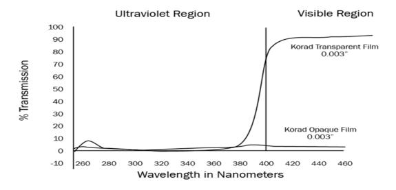
Korad™ Acrylic transparent and pigmented (opaque) films protect thermoplastic substrate by blocking the damaging UV wavelengths of sunlight.
