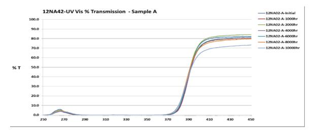
Virtually no UV radiation in the critical range of 295-370 nanometers passes through either transparent or pigmented opaque Korad™ film. The appearance of your Korad™ laminated part will exhibit excellent long-term resistance to fading, crazing, dulling and hazing.
